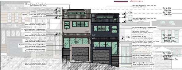
Figure 4: Proposed Rear (East) Elevation at No. 223 Elswick Street North.
