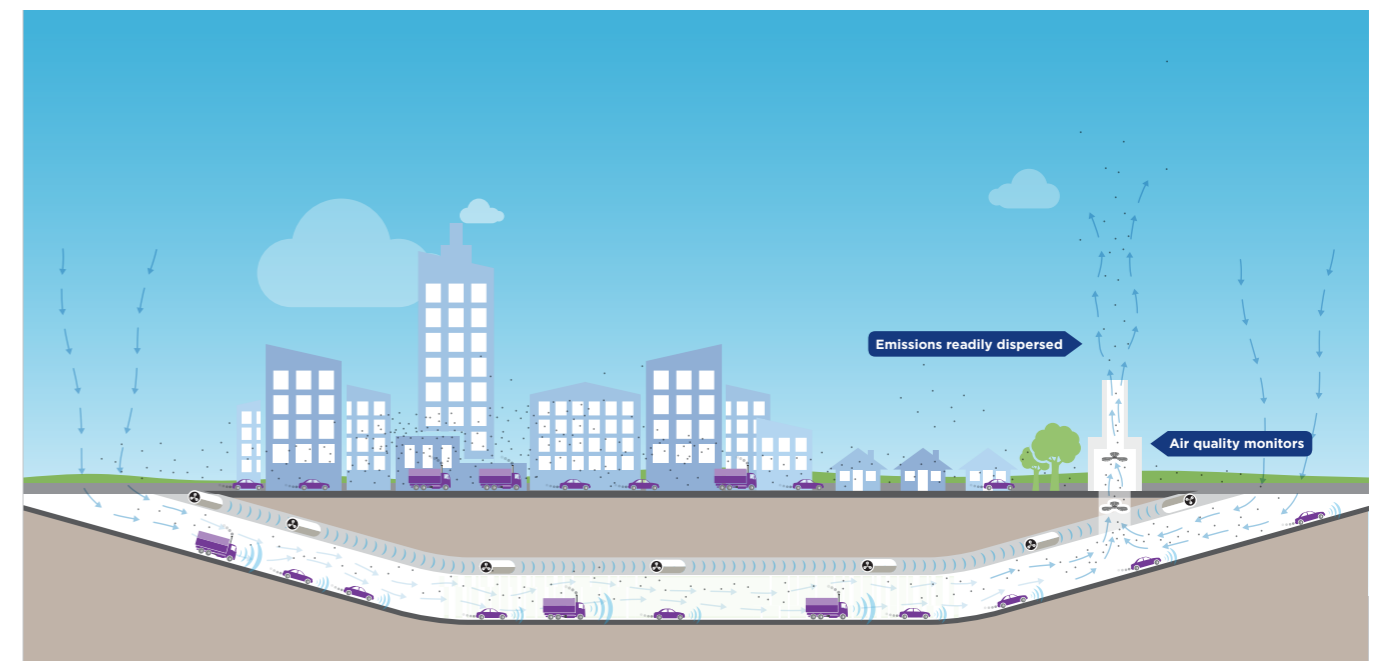
Artist's impression longitudinal tunnel ventilation system
