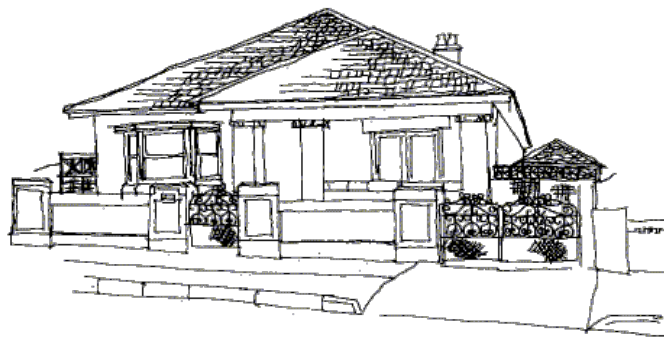
An example of an original low front fence and gate and side boundary fences and gates. Corner blocks traditionally had timber paling fences increasing in height from behind the front building line.
