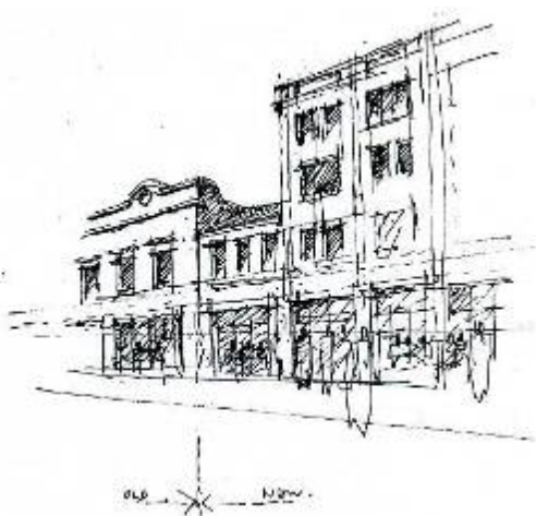
Development adjacent to important parapet corner return Option 1- infill building with pitched roof to retain existing building's visibility.
