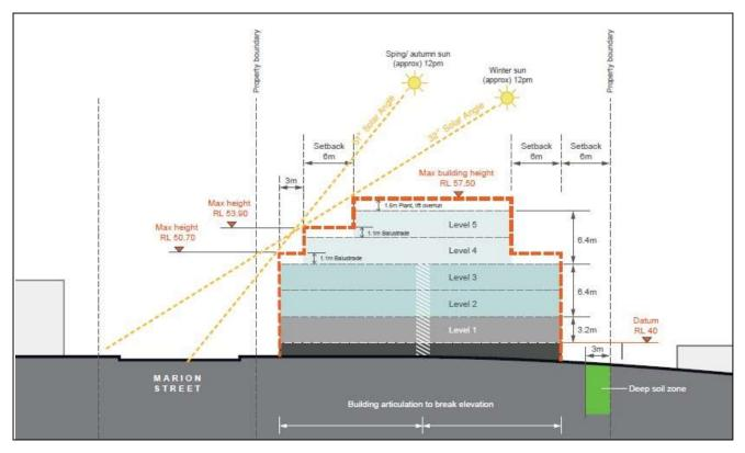
Figure G51: Building Heights and Massing Envelope – Section A (north-south)
