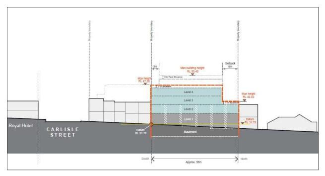
Figure G46: Building heights and Massing envelope - Section A (Norton St elevation)
