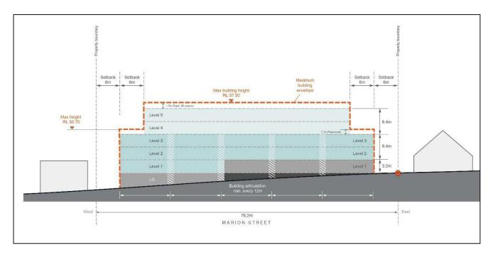
Figure G52: Building Heights and Massing Envelope – Section B (east-west)
