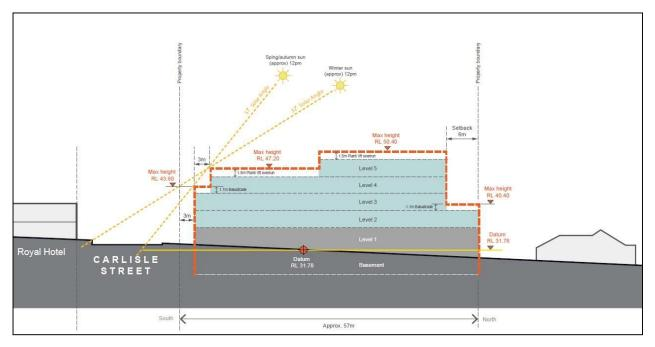
Figure G47: Building heights and Massing envelope - Section C
