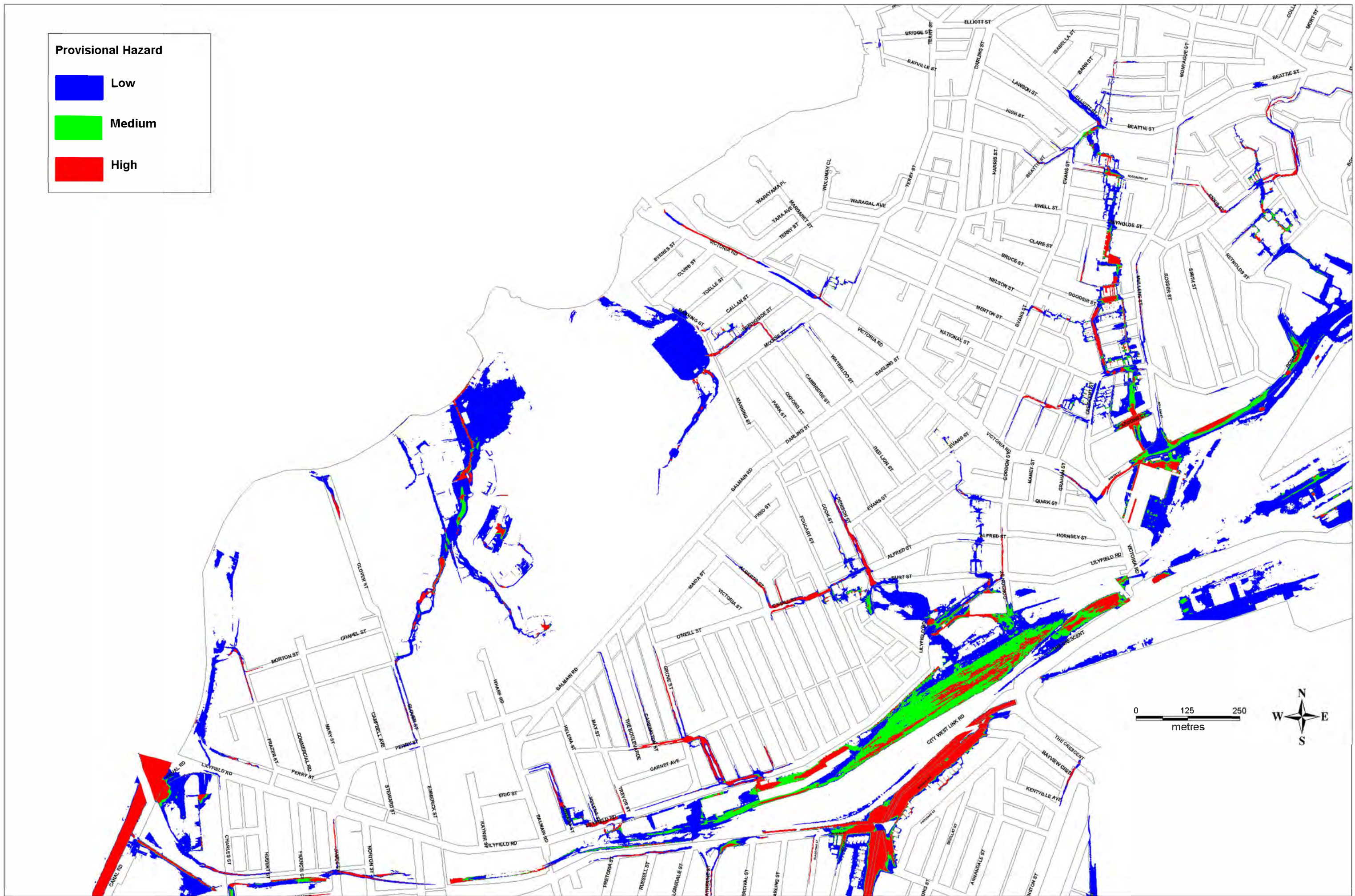
Figure 9.2 - 100yr ARI - Hazard Sheet2
