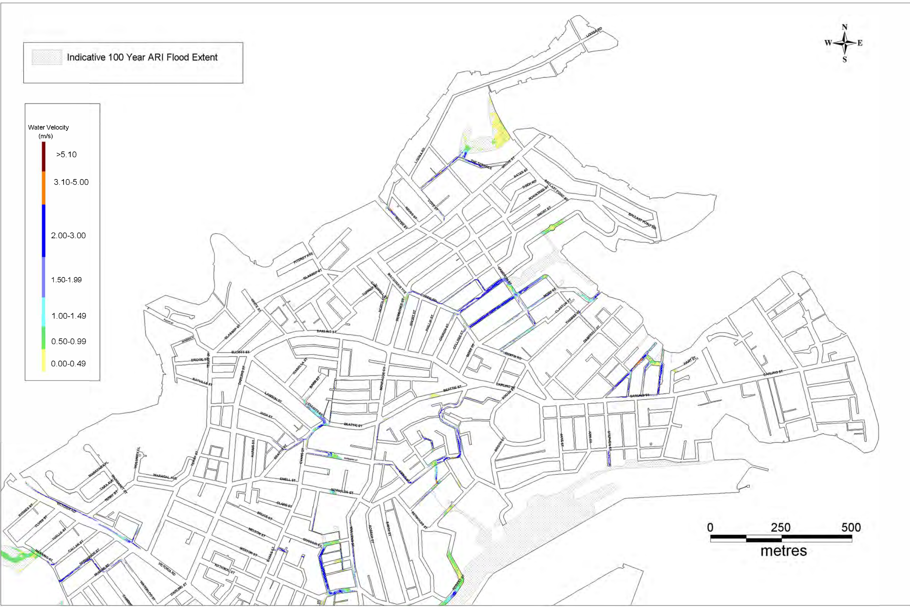
Figure 8.5 - 100yr ARI Peak Velocity Sheet3
