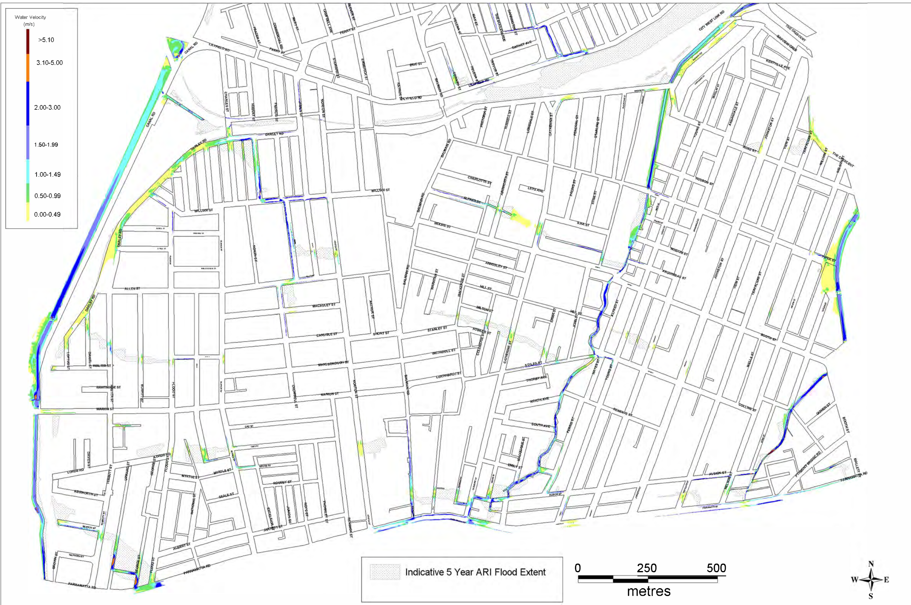
Figure 8.4- 5yr ARI Peak Velocity Sheet1
