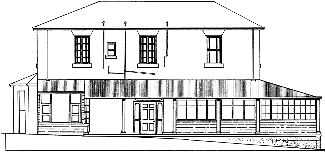
BROUGHTON HALL IN 1984. Situated near the corner of Wharf Road and Church Street the brick and stucco house, in the Georgian Simplified Classical Style, has been drastically altered inside and out. The side verandah was added after 1865.
