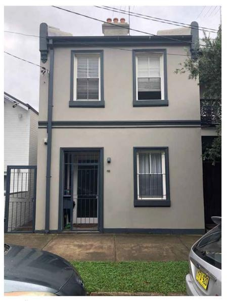
**Figure 5** View of the terrace in Ferris Street. The existing front elevation is not original: the entry opening and windows with their architrave surrounds, the string course and the poorly proportioned window sills are bad attempts at faux heritage. Only the chimney and the parapet ends indicate original fabric.
