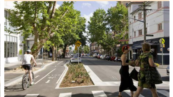
Bourke Street Cycleway is a 3.4 km active transport corridor across a traffic-congested area of inner city Sydney consisting of dense planting, and separate cycleways.
