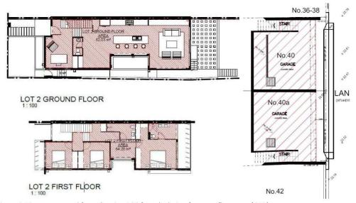
Figure 2 Diagram sourced from drawing A06 for calculation for gross floor area (GFA)
