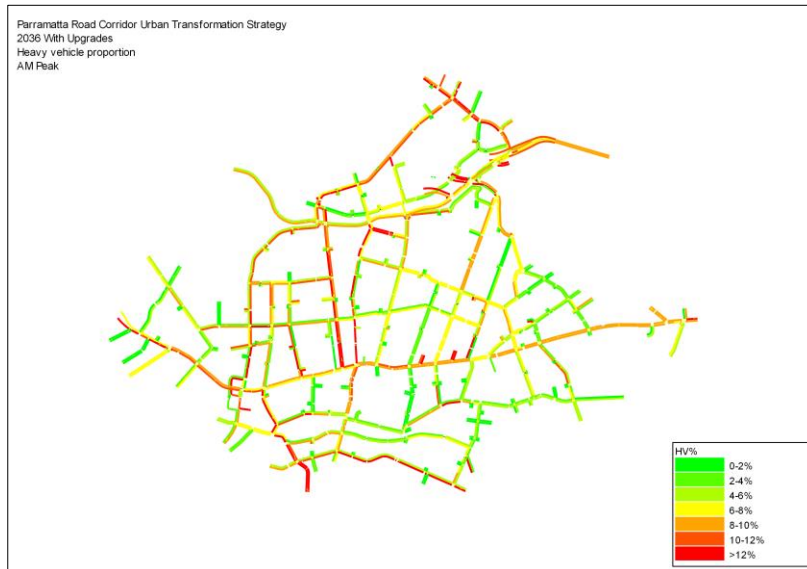
Figure 7-19 Heavy vehicle proportions – 2036 With Upgrades (AM Peak)
