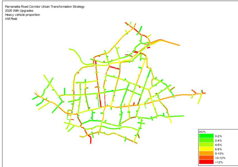
Figure 7-17 Heavy vehicle proportions – 2026 With Upgrades (AM Peak)
