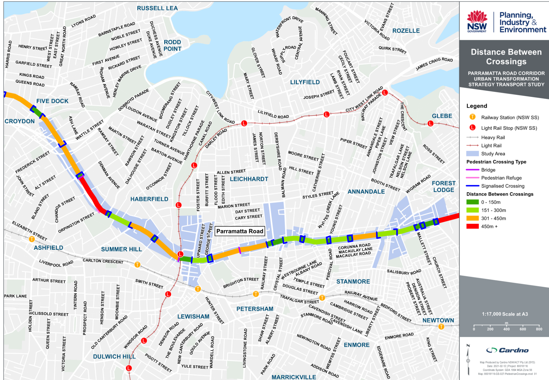
Figure 12-2 Distance between formal pedestrian crossings along Parramatta Road
