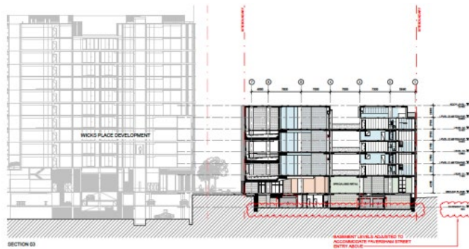
Figure 3 Subject site – Section – Faversham St to Wicks Place, development interface (Place Studio)
