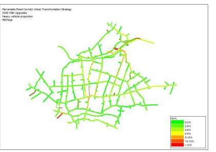
Figure 7-18 Heavy vehicle proportions – 2026 With Upgrades (PM Peak)
