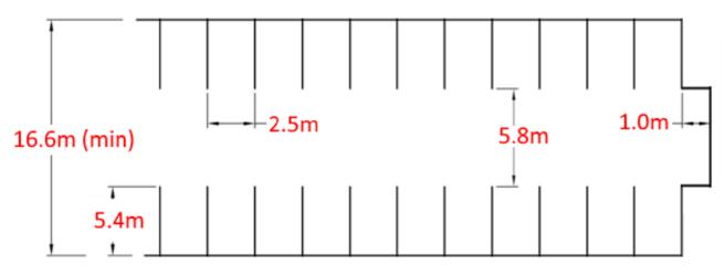
This design gives a minimum floorplate dimension of 16.6m, below which parking cannot be supplied in an efficient manner. For example, a single-sided aisle requires approximately 40% more area per bay, with an equivalent cost increase.
