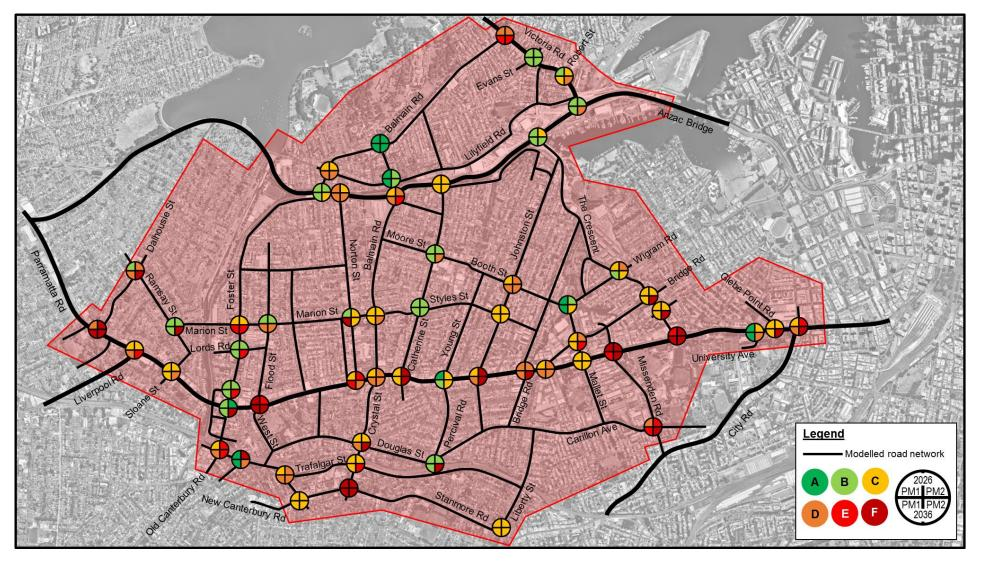
Figure 6-8 Intersection level of service – Do Minimum (PM Peak)
