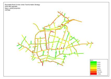
Figure 7-19 Heavy vehicle proportions – 2036 With Upgrades (AM Peak)
