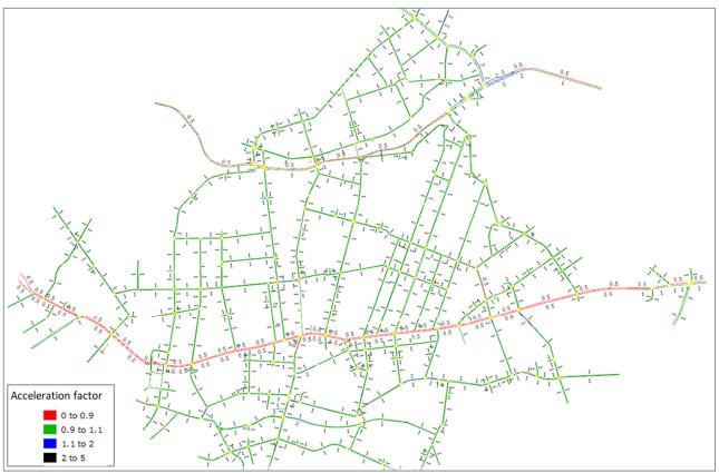
Figure 1: Acceleration factor visualisation of the road network
