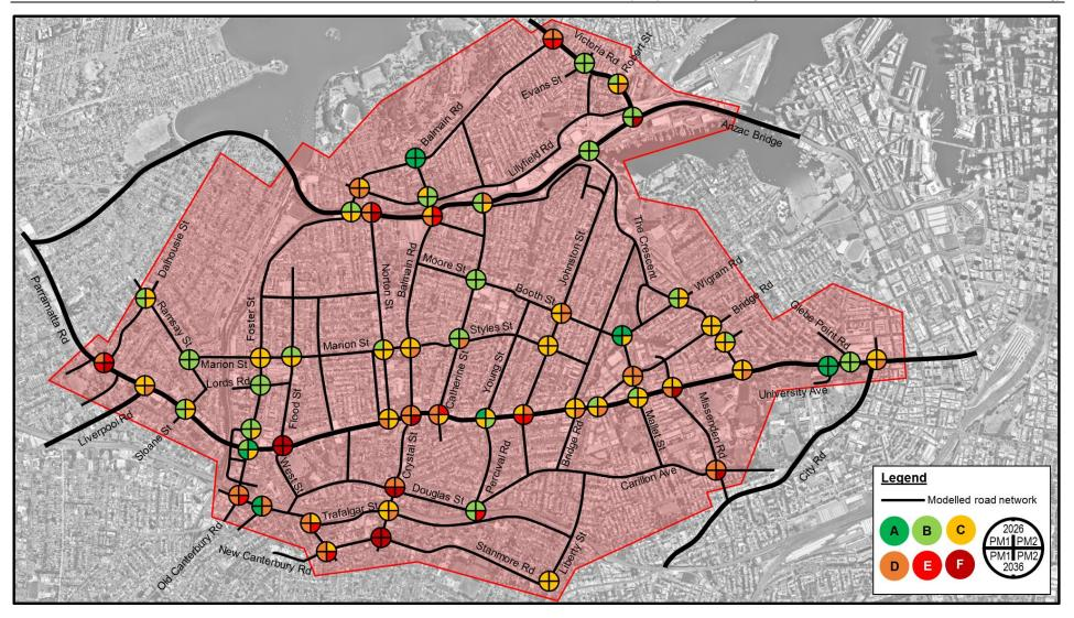
Figure 7-8 Intersection level of service – With Upgrades (PM Peak)
