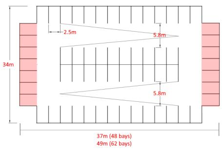
Figure 5-2 Indicative spiral ramp multi-level car park layout
