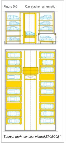
Car stackers are therefore used primarily for low-intensity functions (residential use).
