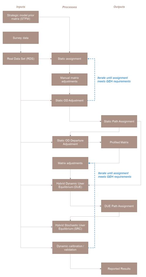
Figure 3-12 Multi-level modelling framework process
