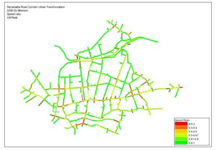
Figure 6-15 Speed ratio – 2036 Do Minimum (AM Peak)
