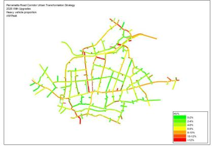
Figure 7-17 Heavy vehicle proportions – 2026 With Upgrades (AM Peak)
