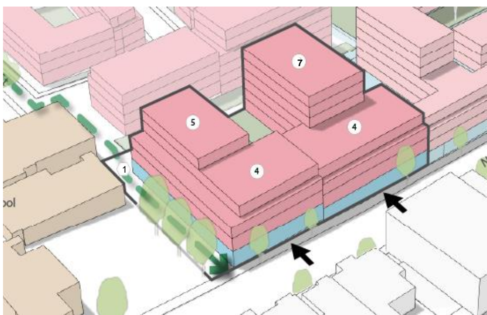
Figure 19: Indicative Area 5: Norton Street North built form bulk, scale and site layout – axonometric and plan view
