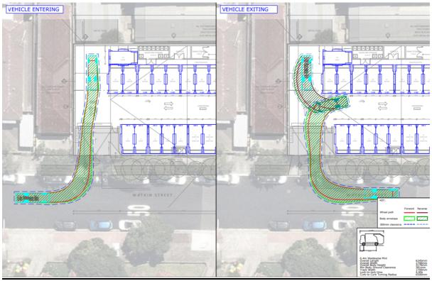
Figure 3: Swept Path diagrams for waste collection
