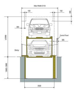
Figure 2: Estimate dimensions for stacked parking system
