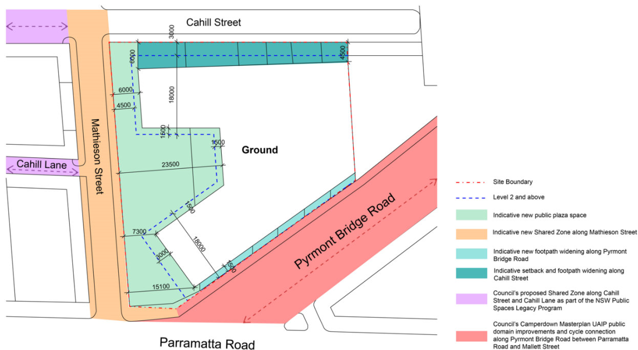
Figure 6 – Indicative revised site plan layout illustrating the proposed setbacks and public domain improvement works
