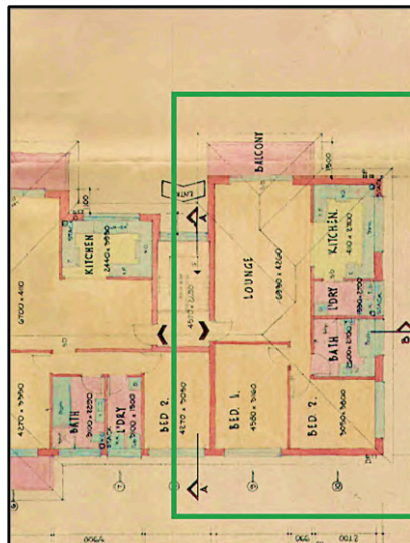
Figure B: Typical unit layout for the ground Level 1 & Level 2. Unit block is angled to the boundary and receives sun to its façade as shown in the sun eye diagrams.
