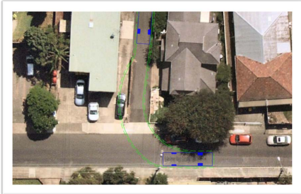
Figure 5 – Swept Paths for Council Garbage truck – turning from Norton Street onto Milton Lane
