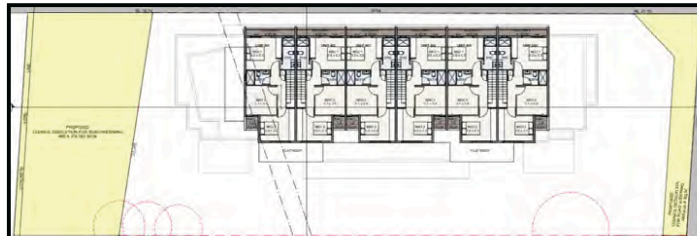
Fig AA - Upper level floor plate provides a 14.435m setback to southern neighbour's wall
