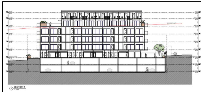
Figure A: Section 1 of the proposed building showing the 12.5m height limit as red dotted line
