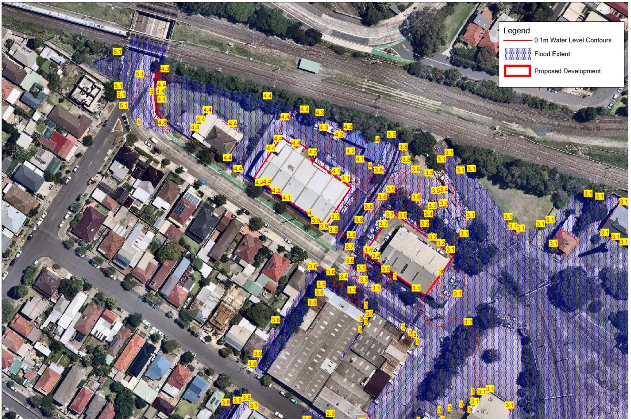
Figure 9 -100yr ARI Flood Level Contours - Future Conditions
