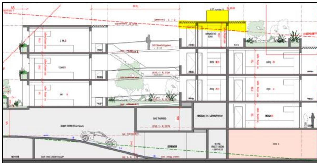
Image 3: Yellow Shaded area demonstrating extent of non-compliance on level 5 and lift-overrun in section.
