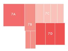
Building 7A is a single storey structure that abuts both north and west boundaries of the site. The north facade of the structure fronts onto Edith St. The structure is comprised of two separate parts, each with a skill ion roof. There is a courtyard on the south side of the building, which houses a sub-station.
