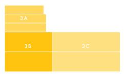
Building 3A is a single storey lightweight structure. The structure has a gable roof on its southern portion and a skillion roof to the north. The building is essentially a 'lean-to', whereby its southern side is supported by the adjacent brick wall from Building 3B.
