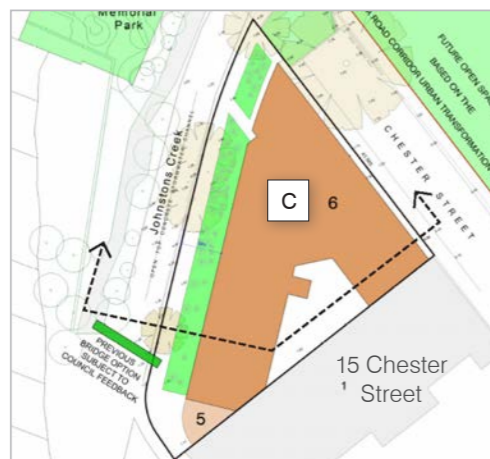
Plan of section cut location showing continuous 6 storey perimeter building and 0m separation at south of site to adjacent site (15 Chester Street) (Extracts from Urban Design Report May 2019 by ae design partnership)
