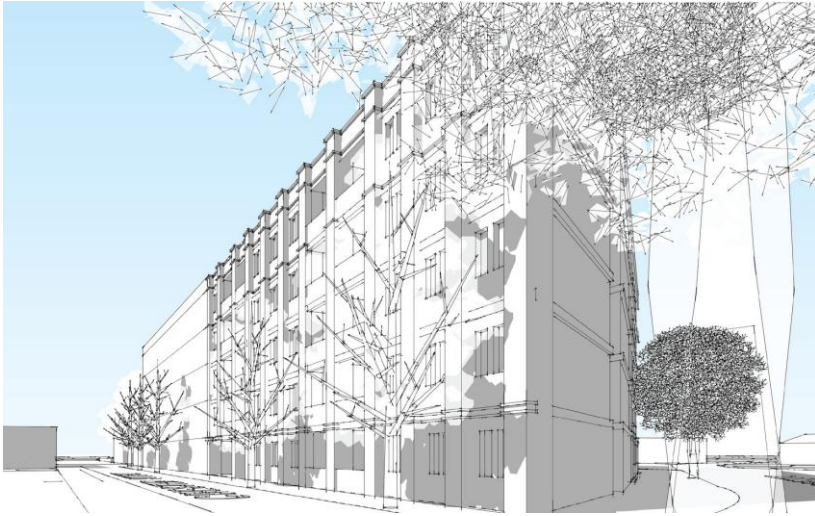
Figure 2: View south to potential design outcome, including appropriate façade treatment emphasising vertical rhythm
