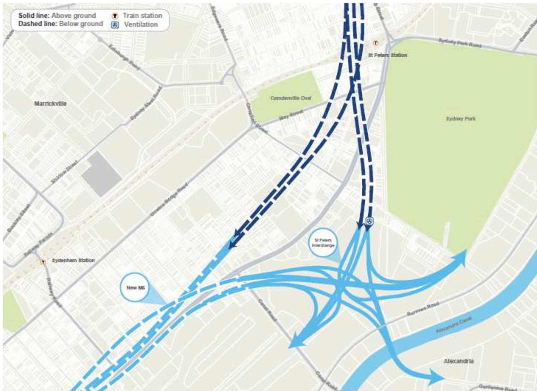
Figure 2.2 St Peters Interchange connections (Source: M4 – M5 Link Concept Design Plan – May 2017)
