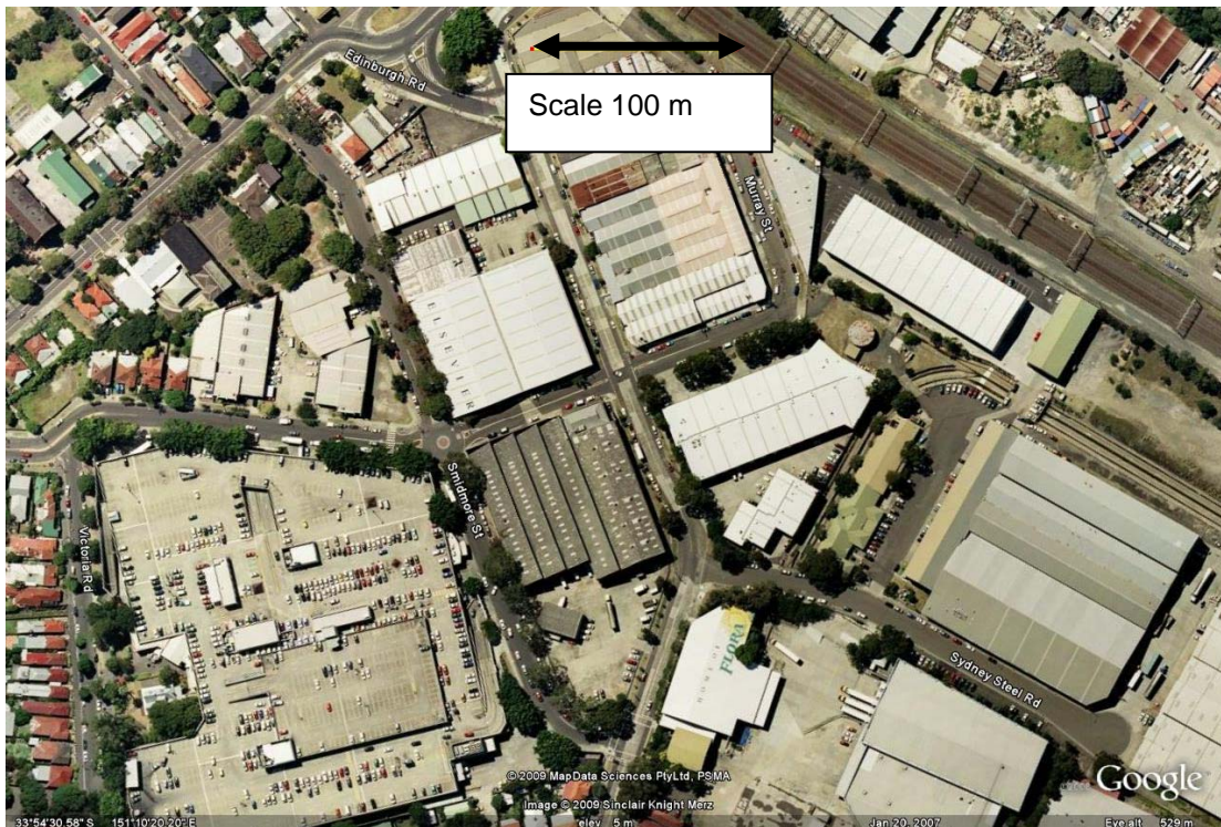
Figure 5: View over Marrickville Metro Shopping Centre and surrounding lands. The shopping centre and the industrial lands have <5% pervious surface. The significant open spaces include school grounds and lands adjacent to the railway. (Image source Google Earth ®)
