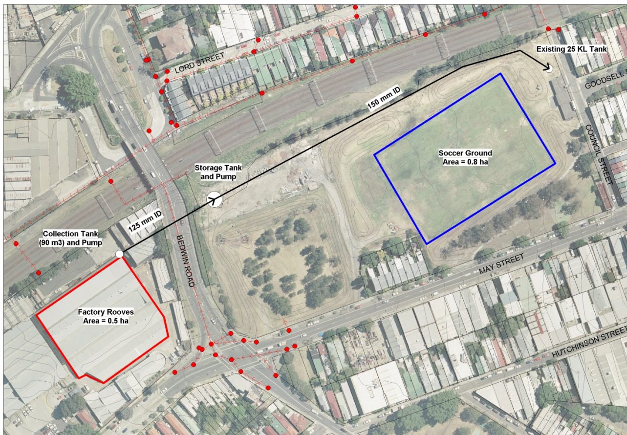
Figure 22: Pipeline route and proposed tank locations.
