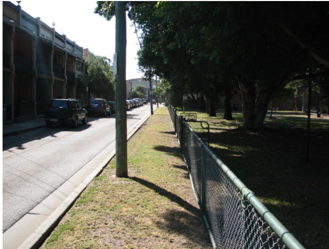
Figure 11: Stormwater is currently conveyed in gutters parallel to the park boundaries. Ideally the gutter on the left hand side of the picture would also be connected to drain into Simpson Park.
