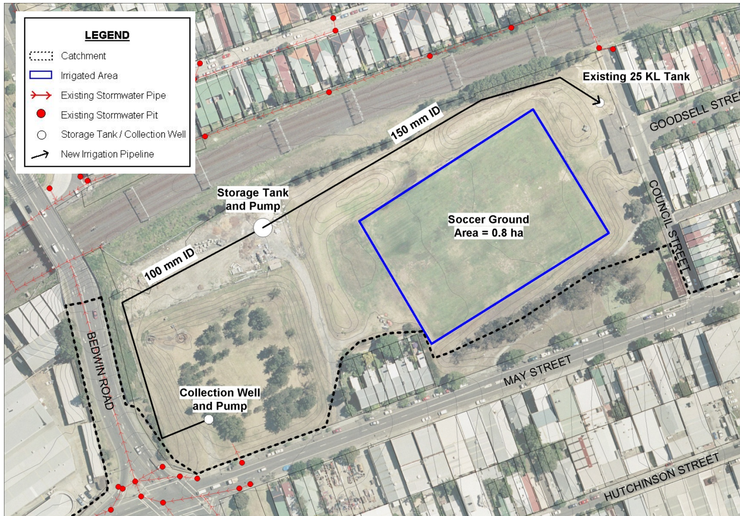
Figure 40: The proposed layout of the capture, storage and supply system.
