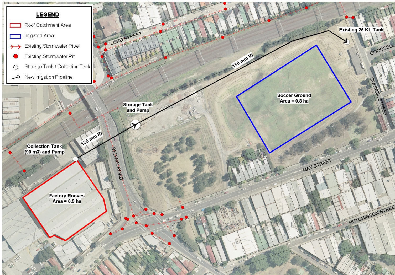
Figure 43: Pipeline route and proposed tank locations.
