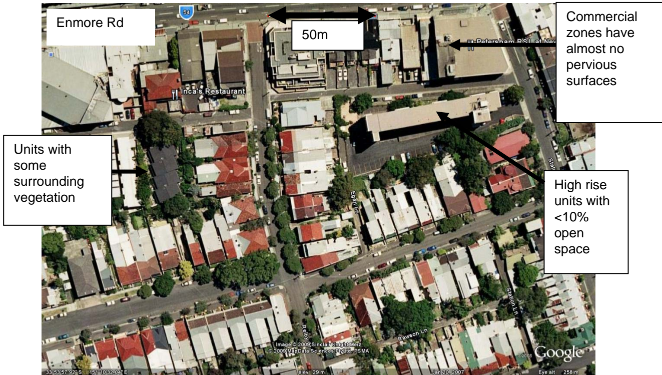
Figure 7: Aerial image of northern portion of catchment. Note lack of 'greenery' behind the commercial strip along Enmore Rd. Street trees are the most obvious vegetation among the residential areas.
