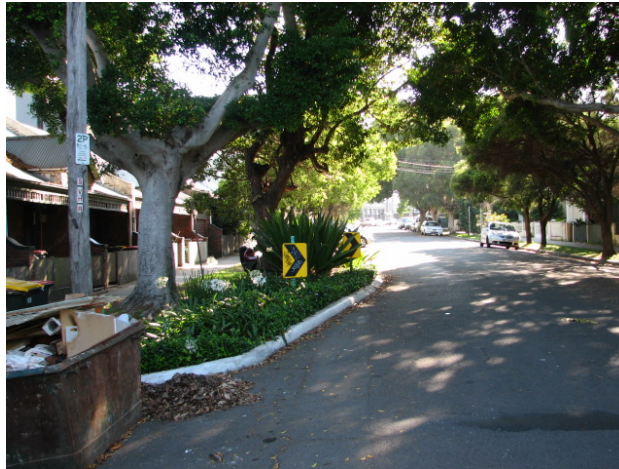
Figure 36: Street gardens could be converted to rain gardens. It would require significant adjustment of levels to enable inflow and discharge of gutter water into the garden.
