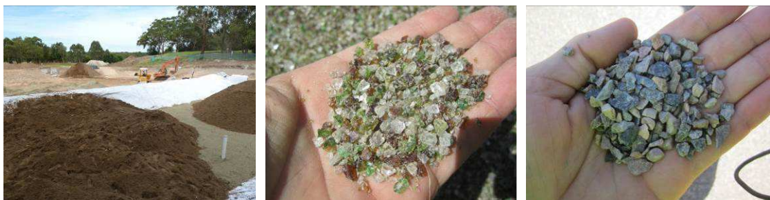
Figure 4 Rain garden media (filter media (sandy loam), transition media (coarse glass) and drainage media (gravel) from left to right)
