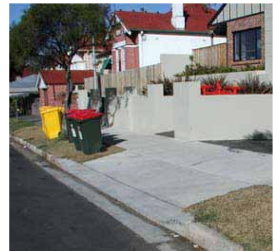
Hard surfaces increase the volume and speed of stormwater runoff that carries pollutants to Cooks River.
