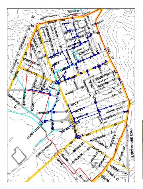
The contour map shows the gradient of the EC East Subcatchment with its ridges and valleys and the locations of the stormwater drainage pits and pipes. The Subcatchment has moderate grades from the ridgelines to the lower areas on the western side of the EC East Subcatchment.
