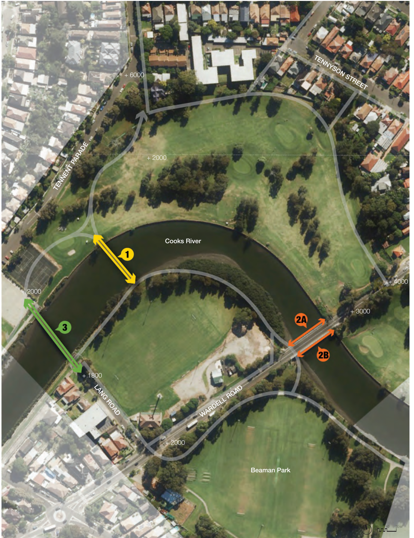
● Option 1 - new bridge ● Option 2 - new separated bridge ● Option 3 - upgrade to existing bridge
